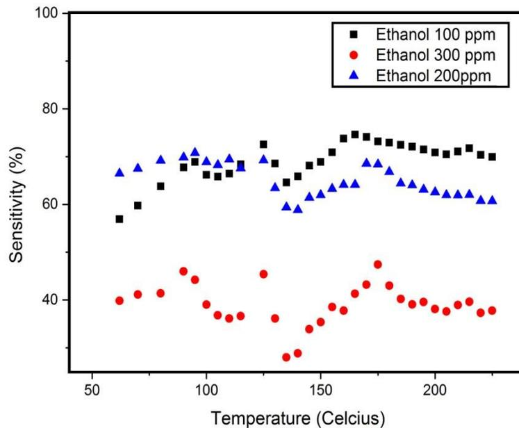
**Figure 6.** Interpretation of thick Film  $Mn_{0.5}Fe_{1.5}O_3-Fe_2O_3$  sensitivity
