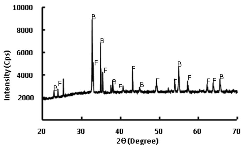
**Figure 4.** XRD pattern of semiconductor ceramic  $\text{Mn}_{0.5}\text{Fe}_{1.5}\text{O}_3\text{-Fe}_2\text{O}_3$ . B is from bixbite, and F is from  $\text{Fe}_2\text{O}_3$ .
