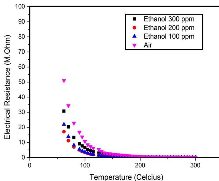
**Figure 5.** The electrical resistance characteristic of thick film  $\text{Mn}_{0.5}\text{Fe}_{1.5}\text{O}_3\text{-Fe}_2\text{O}_3$  to temperature changes.
