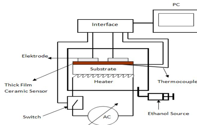
**Figure 2.** The instrument principle for measuring electrical resistance.
