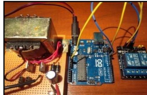
Fig. 4: Connecting Relay with Arduino Uno
