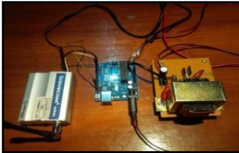
Fig. 6: Assemble SMS Gateway with Arduino
