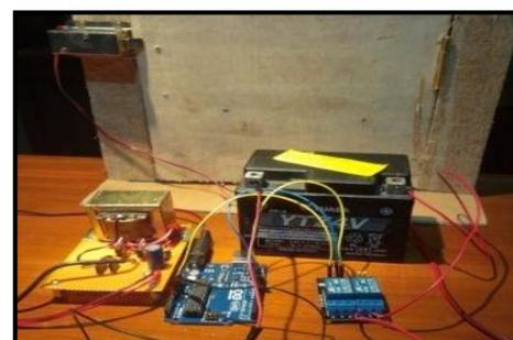
Fig. 5: Assemble Arduino, Solenoid Key, and Relay
