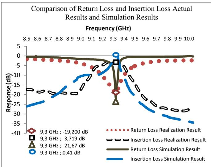
Fig. 6. Comparison of Return Loss and Insertion Loss Actual Results and Simulation Results
