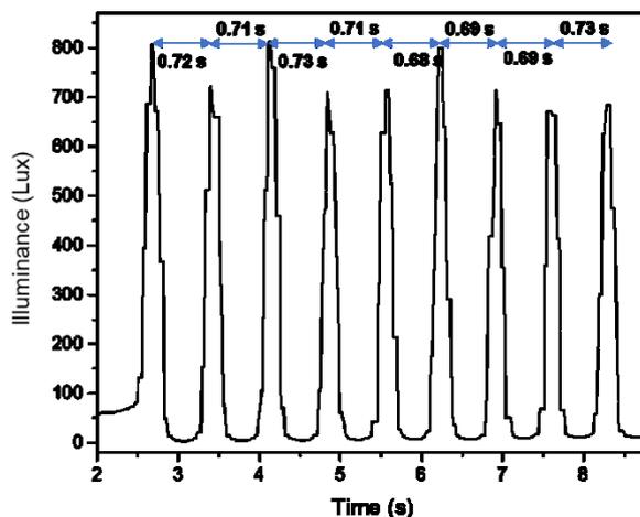
Fig. 4. Curve of light intensity of smartphone.
