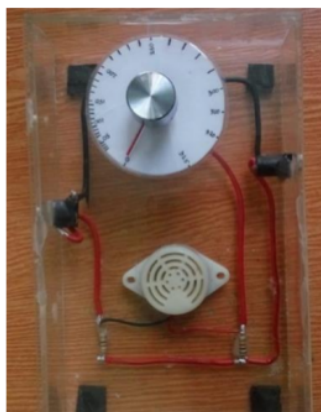
Figure 5. Display of electrolyte solution conductivity measuring device.
