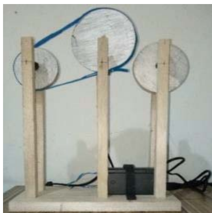
FIGURE 1. Practicum tool to analyze the angular speed and direction of the wheel's movement
