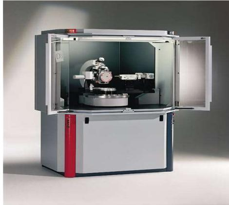
**Gambar 3. 6** Peralatan X-Ray Diffractometry [33].
