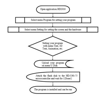
Figure 4. Flowchart of programing and installing videotron
