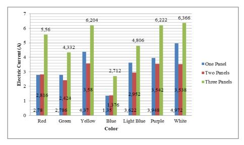
Figure 5. Data from the measurement of electric current in panel P.6 videotron with different background color
