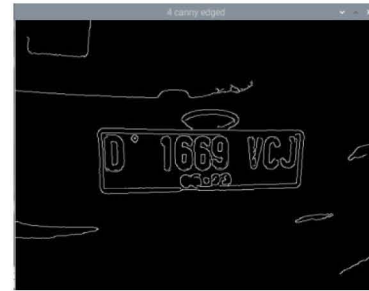
Fig 5. Edge detection with Otsu Thresholding method
