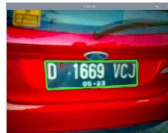
Fig 6. The bounding box from edge detection
