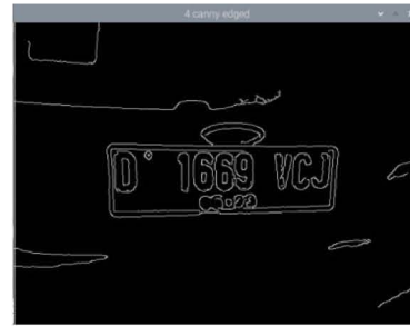
Fig 4. Edge detection with Canny Edge method
