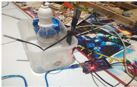
Fig. 11. Relay and temperature sensor DS18B20 testing
