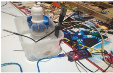
Fig. 11. Relay and temperature sensor DS18B20 testing
