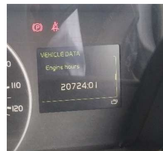
Fig. 1. Hour Meter shows engine has been running for 20724 hours on a FH16 Truck Head
