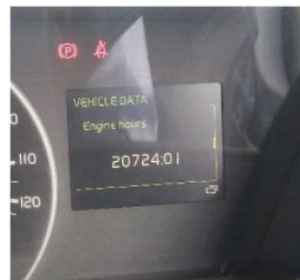
Fig. 1. Hour Meter shows engine has been running for 20724 hours on a FH16 Truck Head
