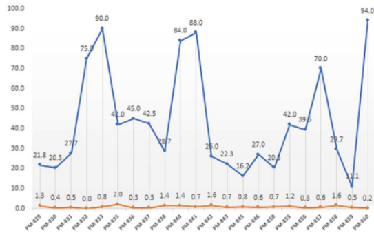
Fig. 11. Graph Showing MTTR (orange line) and MTBF (blue line) of Volvo machine after the implementation of real time precision maintenance scheduler
