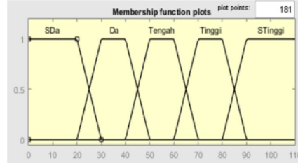
Fig. 3. Membership function of the sensor below
