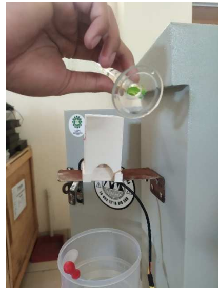
Fig. 12. Process rainfall sensor calibration.
