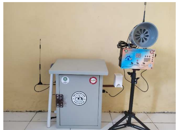
Fig. 7. Sender module system and receiver modul system.
